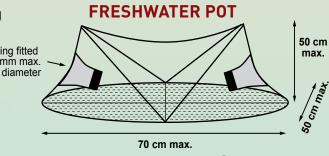
Max. number of openings: 2 15 mm Min. mesh size 15 mm when stretched
